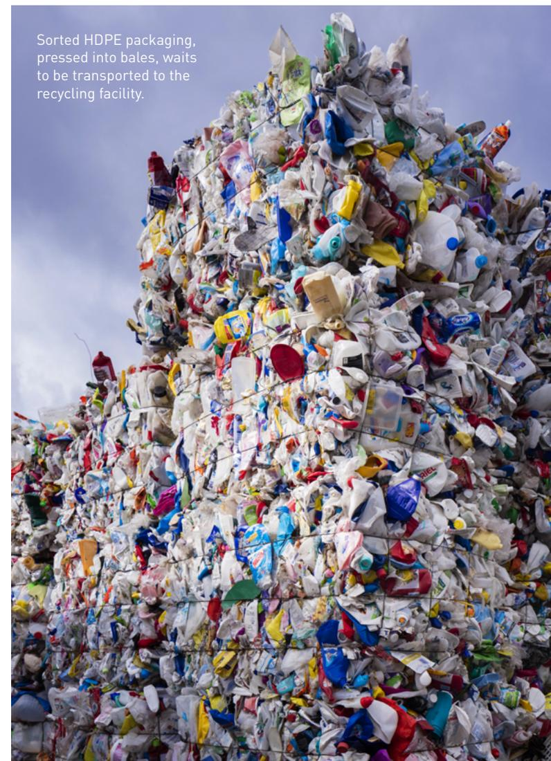
Sorted HDPE packaging, pressed into bales, waits to be transported to the recycling facility.
