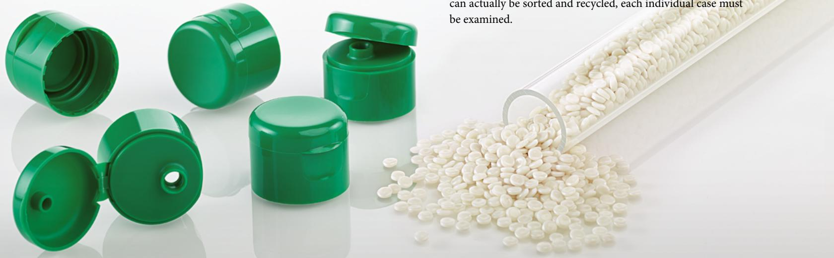
High-quality regranulates for new packaging, e.g., flip-top caps, can be produced from optimally recyclable plastic packaging.
