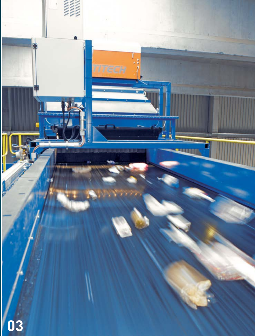
Intelligent technology: near-infrared sorters detect the type of plastic using its reflected light – compressed air ensures maximally accurate separation.
