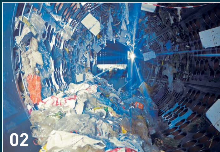
The screen drum separates the packages by size.
