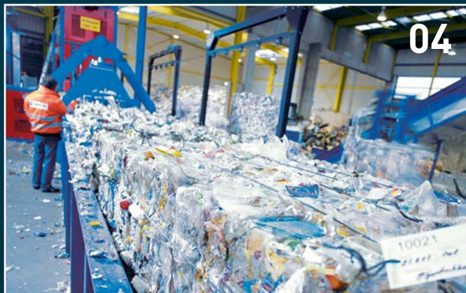
After the recyclables have been separated into many different fractions, the bale press shapes them into blocks of identical size.
